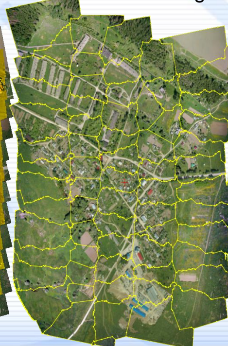
orthomosaic seam lines and color balancing
