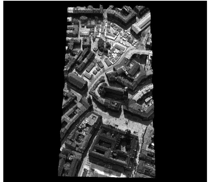
TIN derived from unfiltered point cloud
