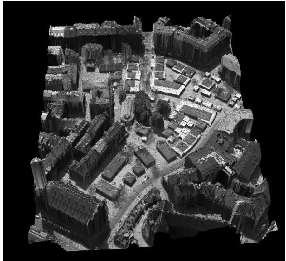
TIN derived from unfiltered point cloud
