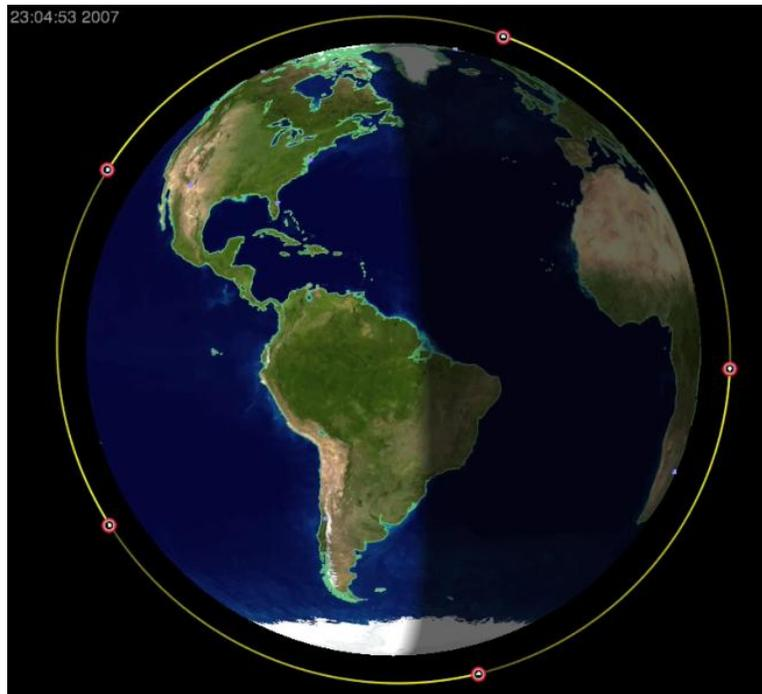
Equally spaced in one orbital plane
