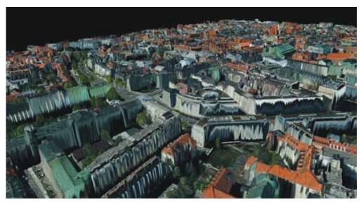
We used orthophoto as a texture – this lead to the building walls not colored correctly. The new DSM module works with aerial and pushbroom images and will be available with PHOTOMOD 6.0 release.
