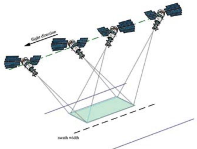
Stereoimaging is performed at a single turn with a deviation by pitch. Length of routes is up to 115 km.
