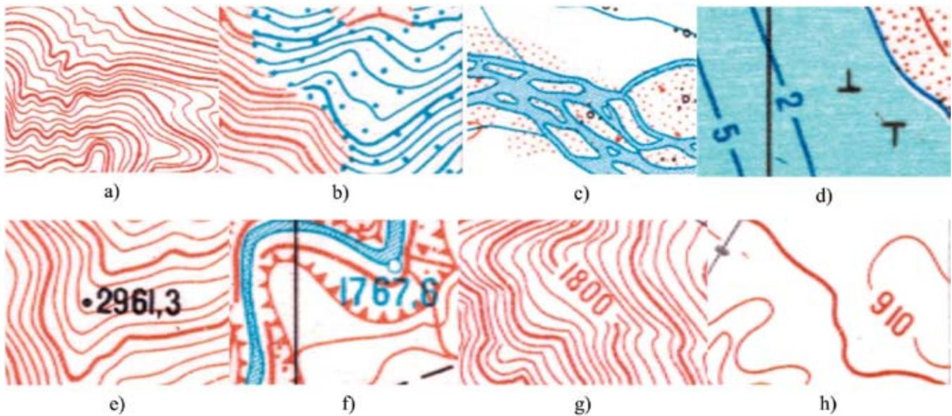
Fig. 1. Main topographic map relief elements
