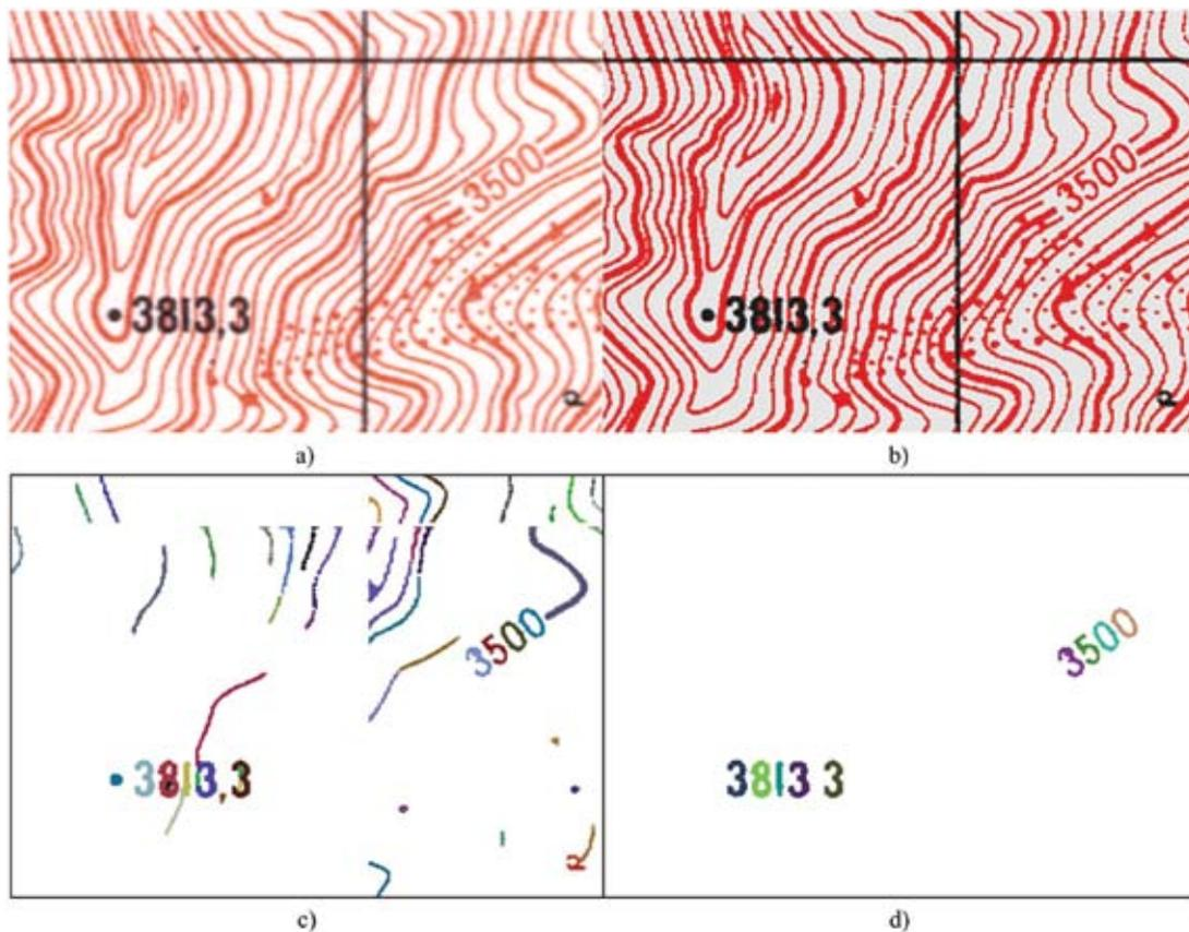
Fig. 3. Source topographic map (a) color segmentation (b), values recognition (c) and numeric sequences creation (d)
