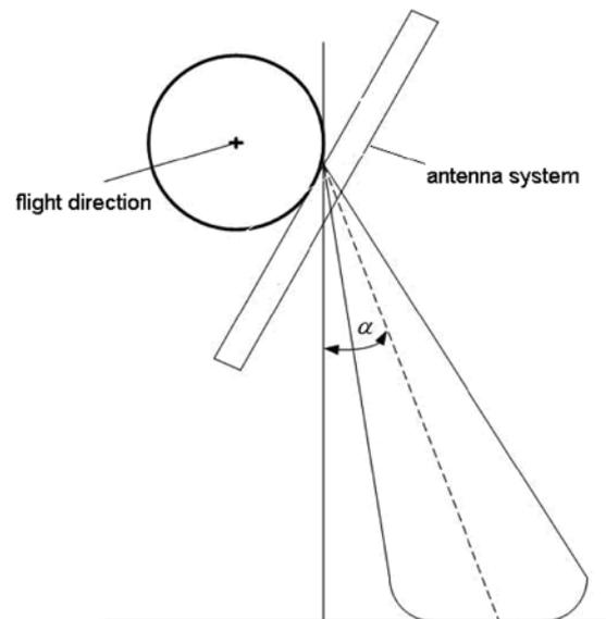
Figure 4: Direction of antenna beam relative to the flight direction of the ISS.
