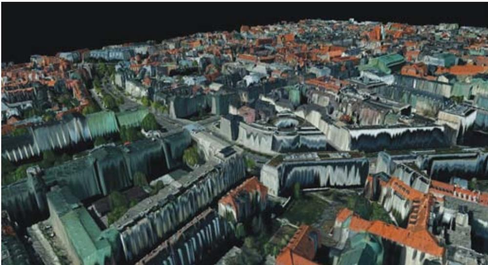
We used orthophoto as a texture – this lead to the building walls not colored correctly. The new DSM module works with aerial and pushbroom
