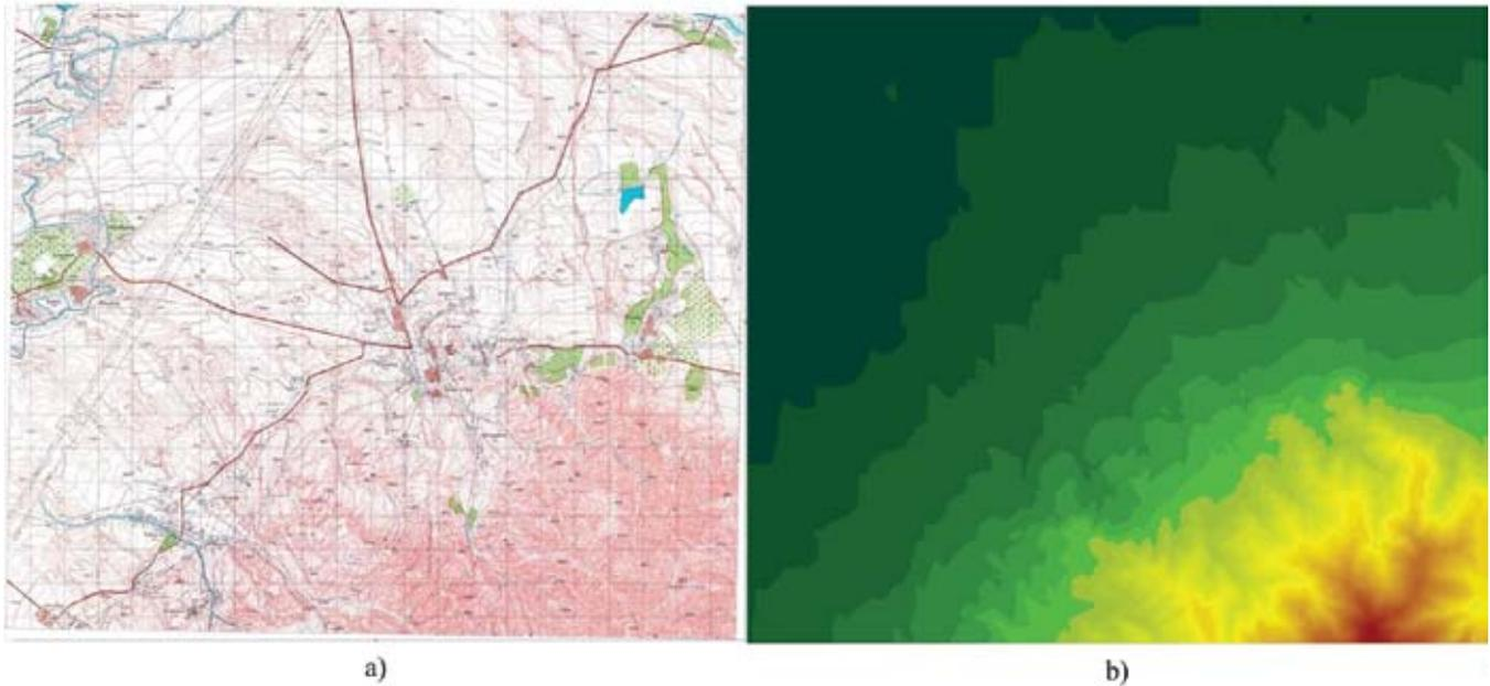
Fig. 4. Regular DEM (b) based on the topographic map (a)
