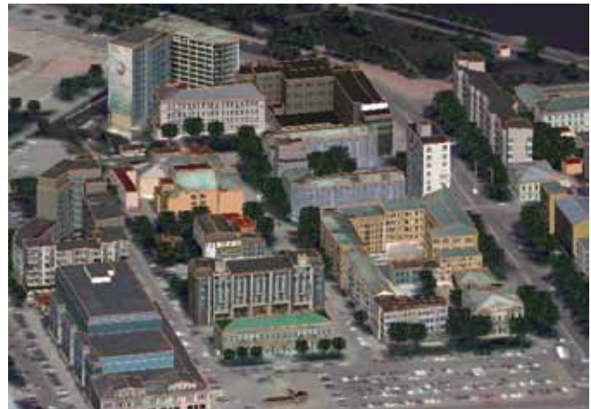
Fig. 2. 3D model on the basis of stereo-photogrammetric processing of satellite images.
