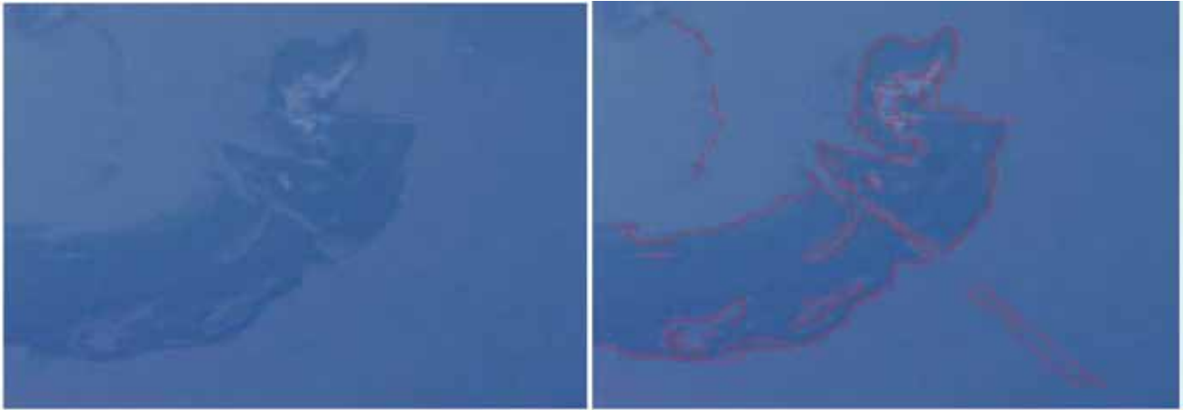
Fig.2. Identification of the boundaries of the spot on the sea surface and the track from the passing vessel
