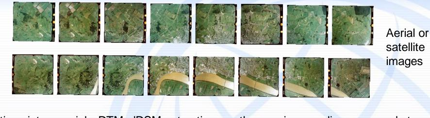
tie points + aerial DTM, dDSM extraction orthomosaic seam lines manual stereo and filtering triangulation and color balancing vectorization
