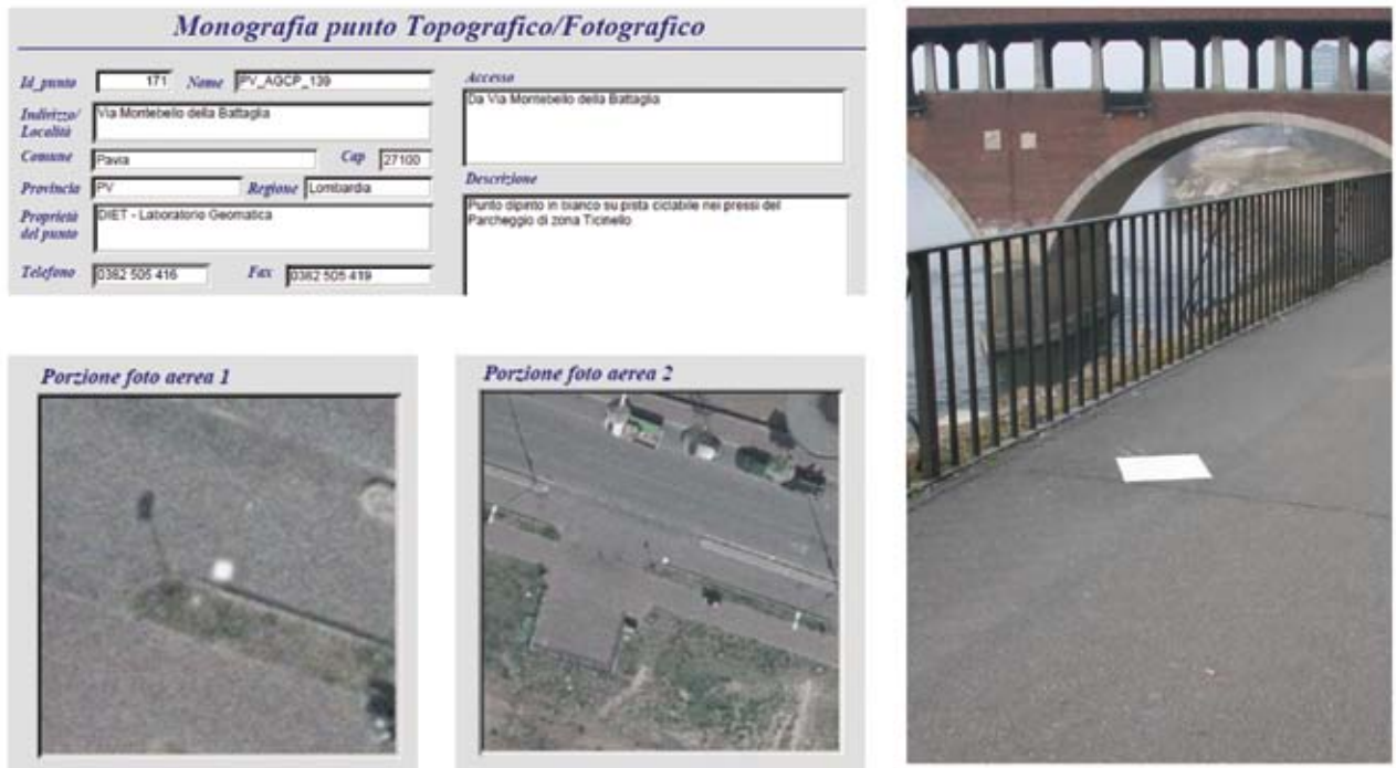
Figure 6. Example of GCP: on the left is shown a portion of the original monography and on the right an image taken on the ground
