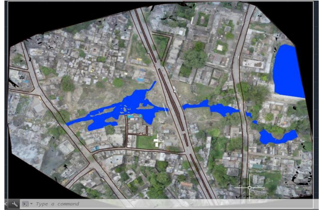
Orthomosaic imported in AutoCAD for digitization of water bodies
