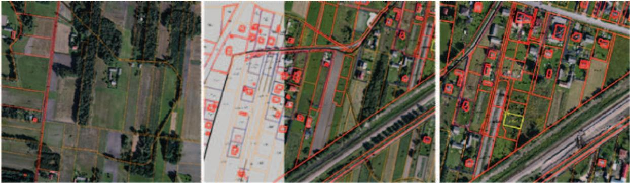
Fig. 2. Orthoimage based on UAV imagery with vector layers of cadastral maps: buildings and plots
